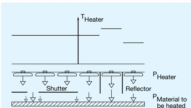
Figure 17: Power adjustment with reflector and shutter
