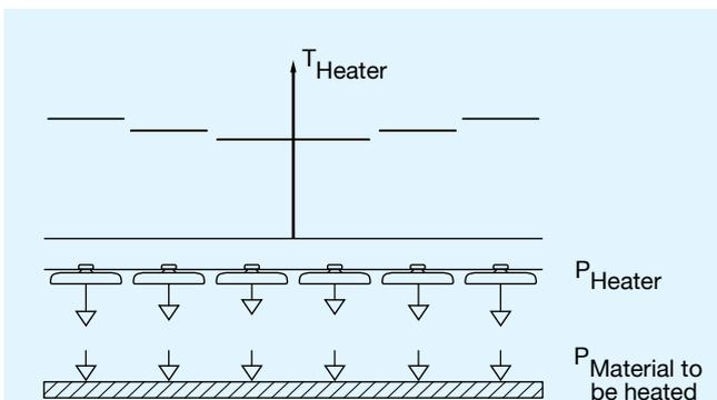
Figure 16: Power at the material to be heated with adjusted heater power
