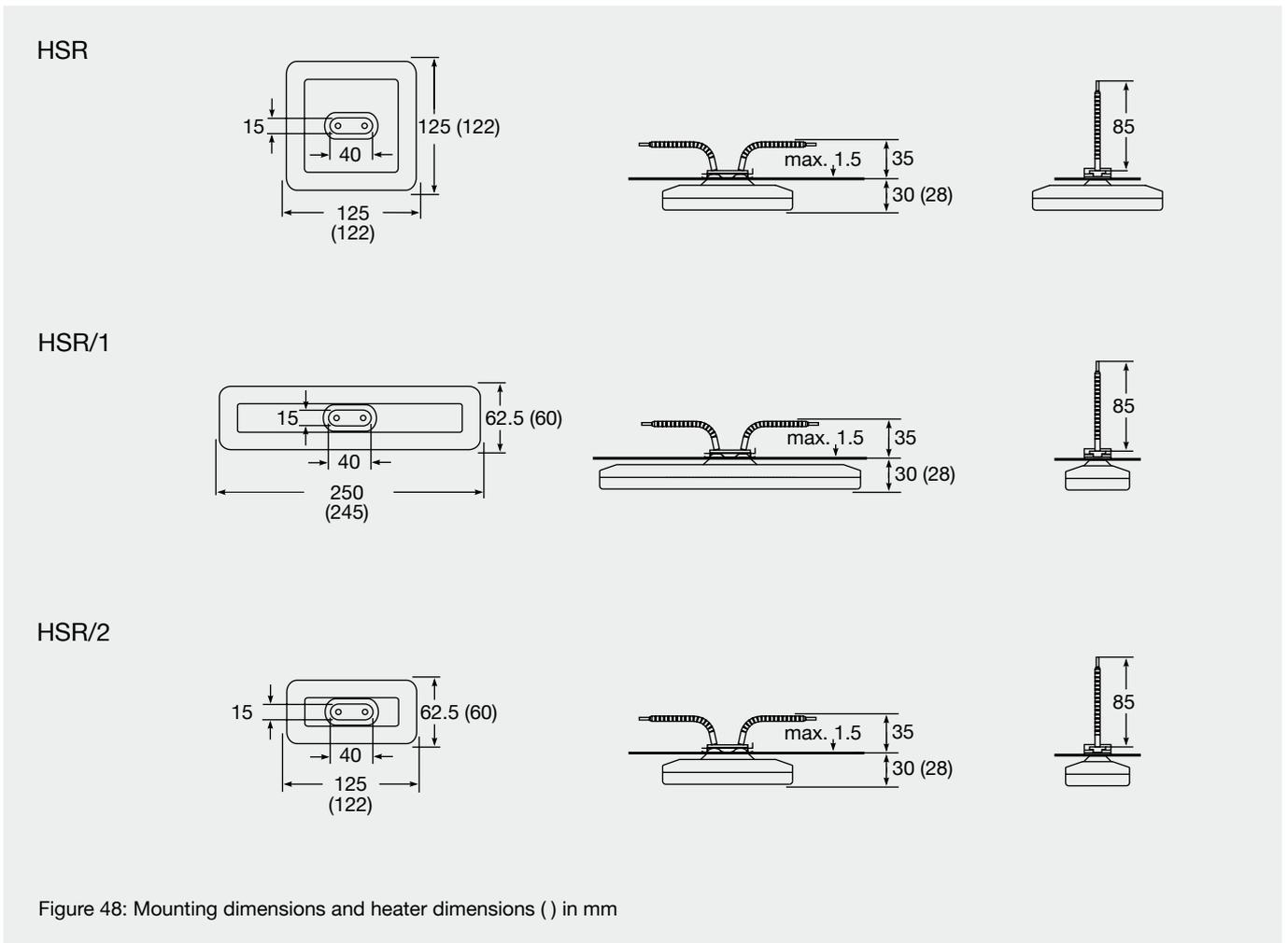
Figure 48: Mounting dimensions and heater dimensions ( ) in mm
