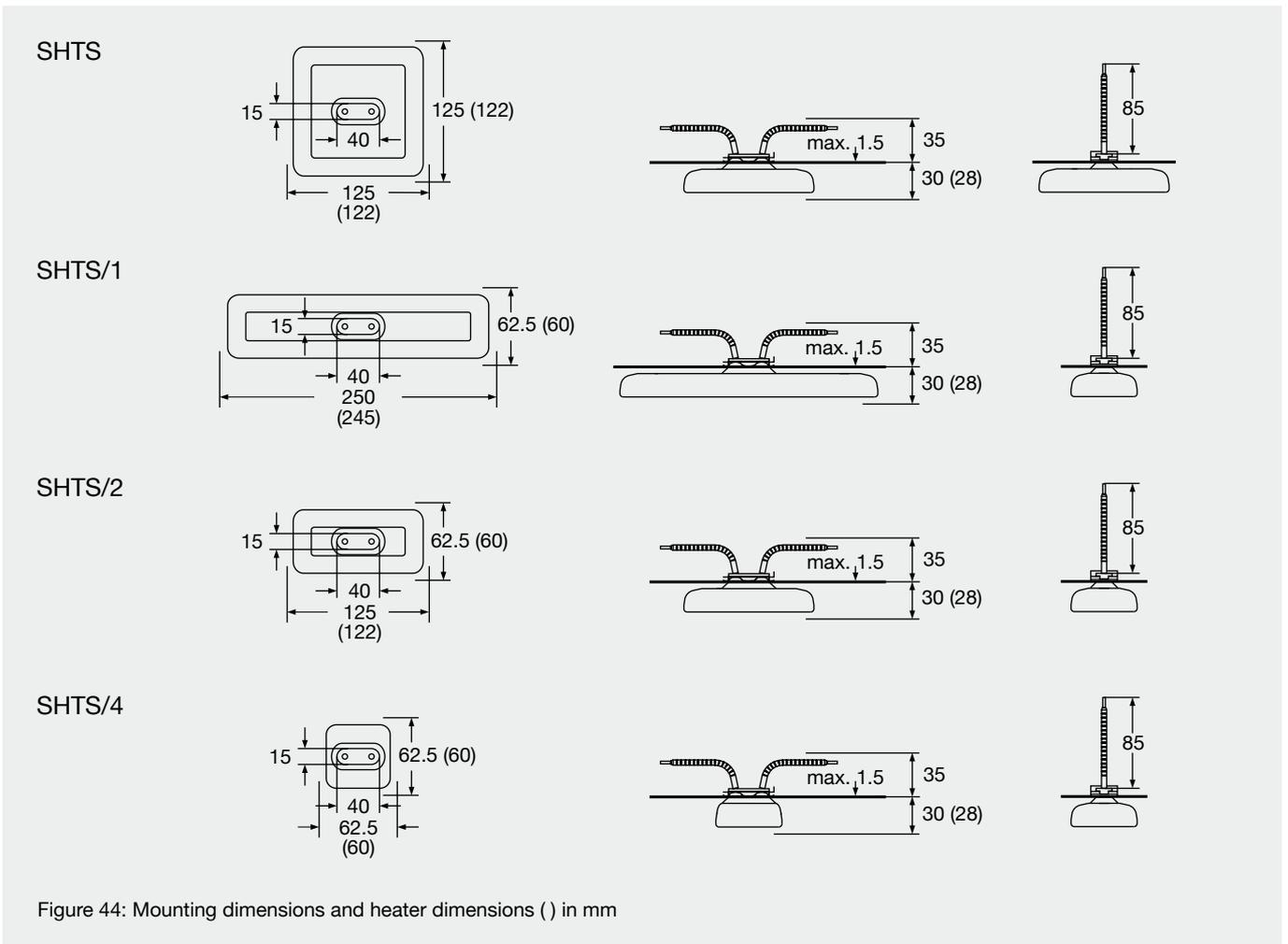
Figure 44: Mounting dimensions and heater dimensions ( ) in mm
