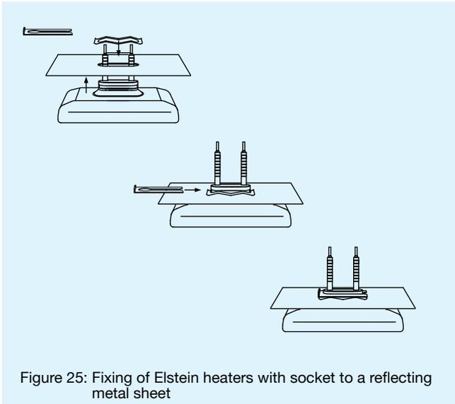
Figure 25: Fixing of Elstein heaters with socket to a reflecting metal sheet
