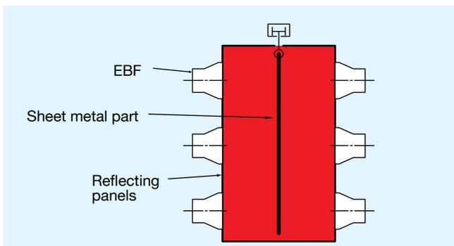
Figure 11: Radiation tunnel with several EBF systems
