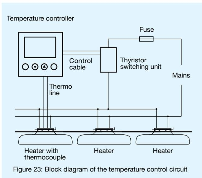
Figure 23: Block diagram of the temperature control circuit
