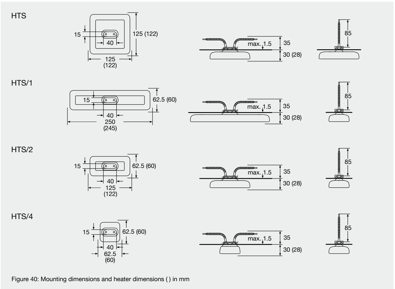
Figure 40: Mounting dimensions and heater dimensions ( ) in mm
