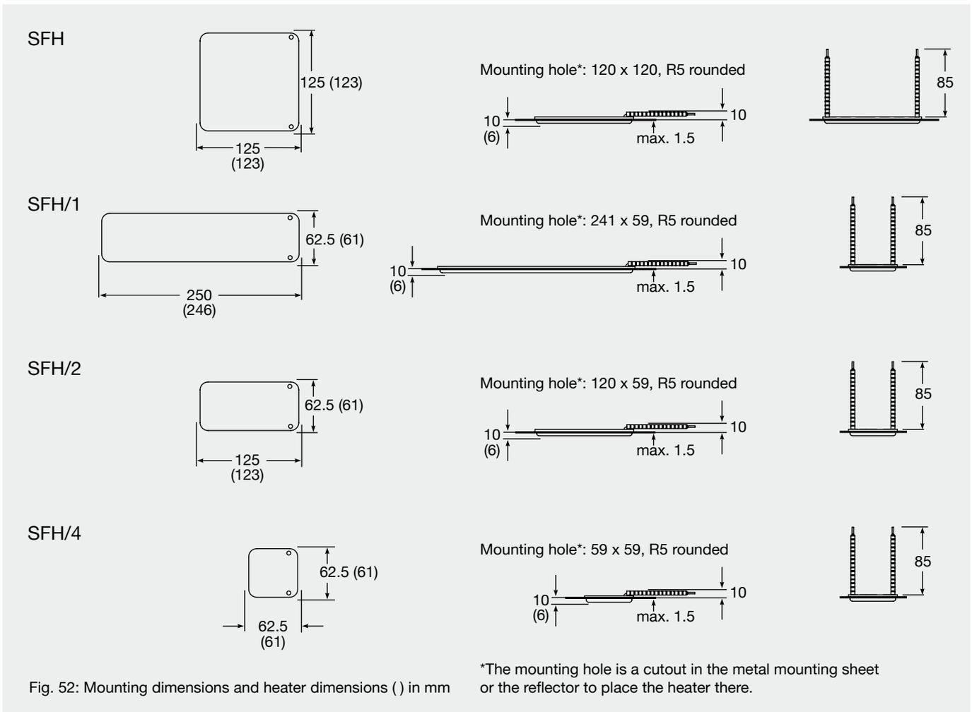
Fig. 52: Mounting dimensions and heater dimensions ( ) in mm
