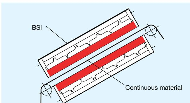
Figure 12: Heating a continuous material using 2 BSI systems
