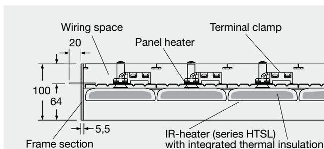
Fig. 89: Structural design of the BSI construction panel
