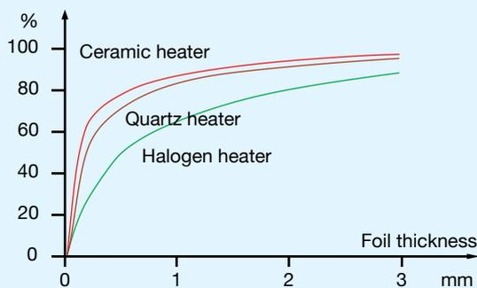
Figure 20: Absorption in transparent foils
