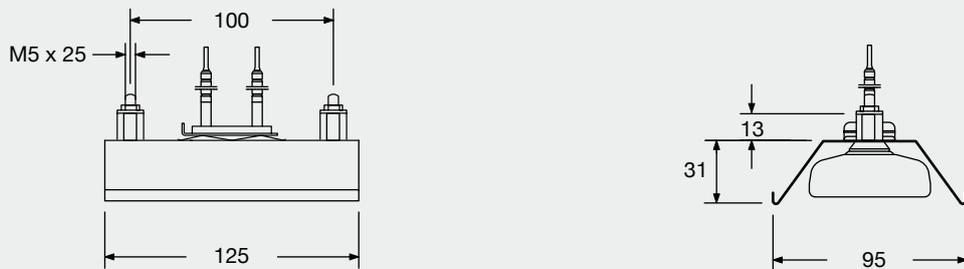
Figure 72: Mounting dimensions and REF dimensions ( ) in mm
