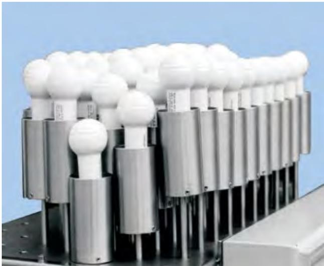
Figure 8: 3-D heating panel for laminating door trims
