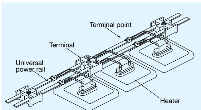
Figure 13: Rail wiring
