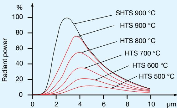
Figure 4: Spectral radiant power of Elstein heaters
