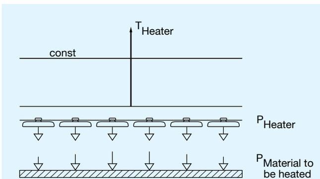
Figure 15: Power at the material to be heated with constant heater power
