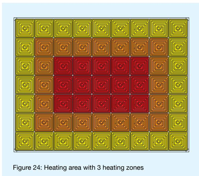
Figure 24: Heating area with 3 heating zones
