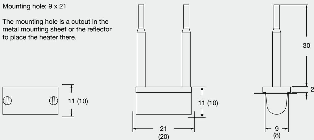
Figure 56: Mounting dimensions and heater dimensions ( ) in mm
