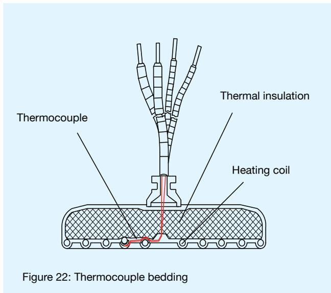
Figure 22: Thermocouple bedding
