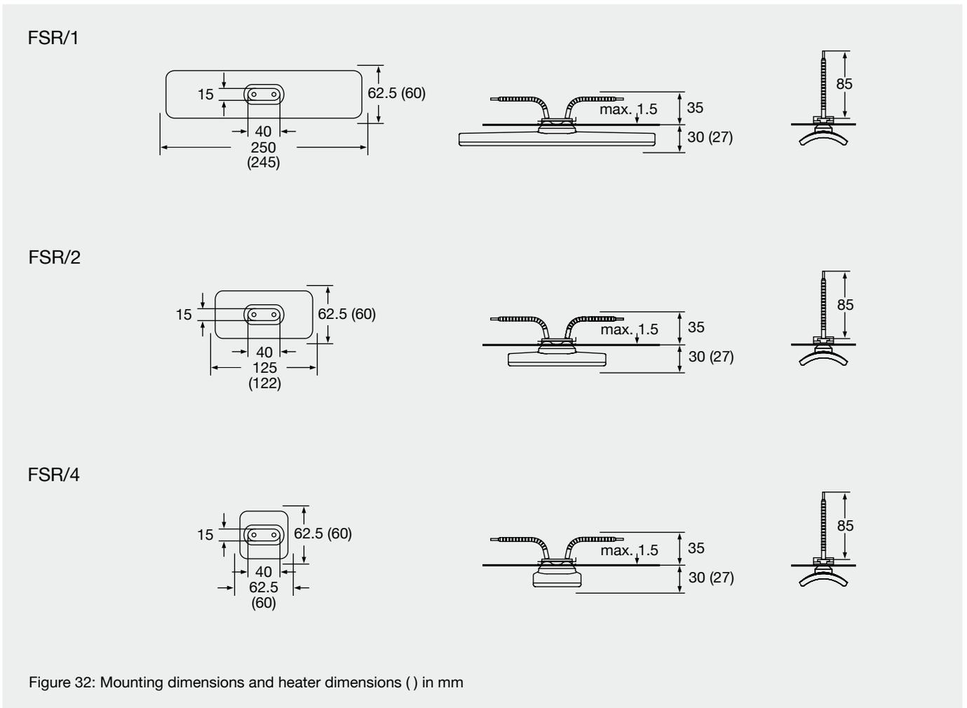
Figure 32: Mounting dimensions and heater dimensions ( ) in mm
