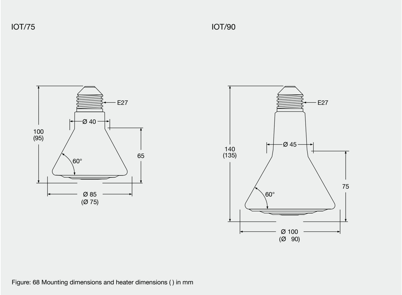
Figure: 68 Mounting dimensions and heater dimensions ( ) in mm
