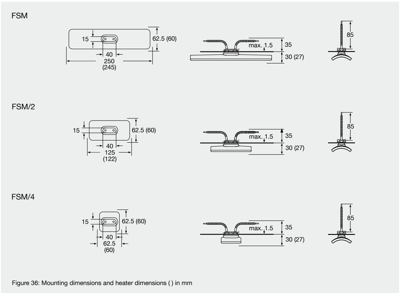
Figure 36: Mounting dimensions and heater dimensions ( ) in mm
