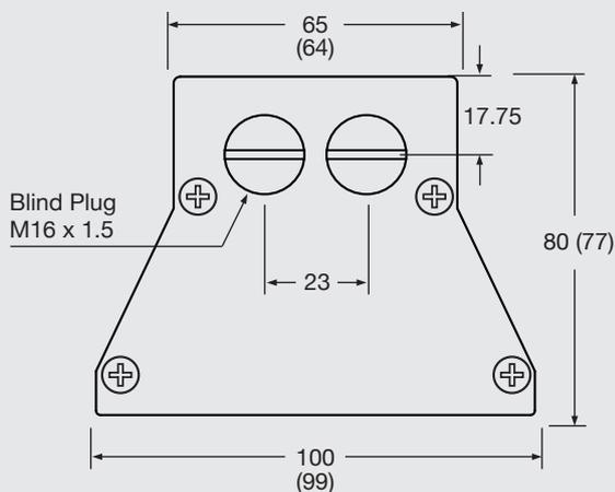
Mounting dimensions and EBF dimensions ( ) in mm
