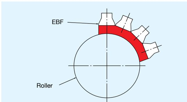
Figure 10: Roller heating using the EBF system
