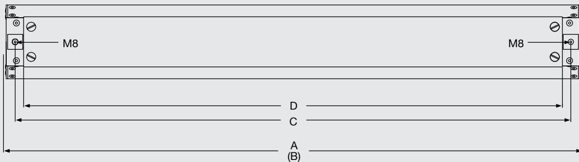
When exchanging EBF against EBI varying dimensions of housing and installation must be considered.
